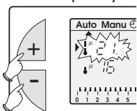
The current temperature level indicator (comfort or reduced) will begin flashing. This modification ends with the next change in programmed temperature. To return to the initial programme press **MODE** and re-position the pointer **▲** under **Auto**. The current temperature level indicator (comfort or reduced) will stop flashing when the temporary modification comes to an end.
