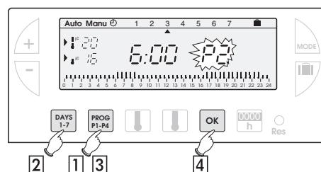
① Press the **PROG P1-P4** button to go into programming mode.
