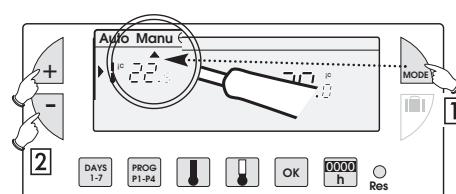
① Press the **MODE** button to position the pointer **▲** under **Manu**.
