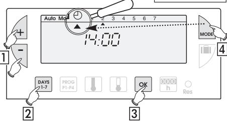
① Set the time using the **+-** buttons (the numbers run off more quickly when the button is pressed continuously).
