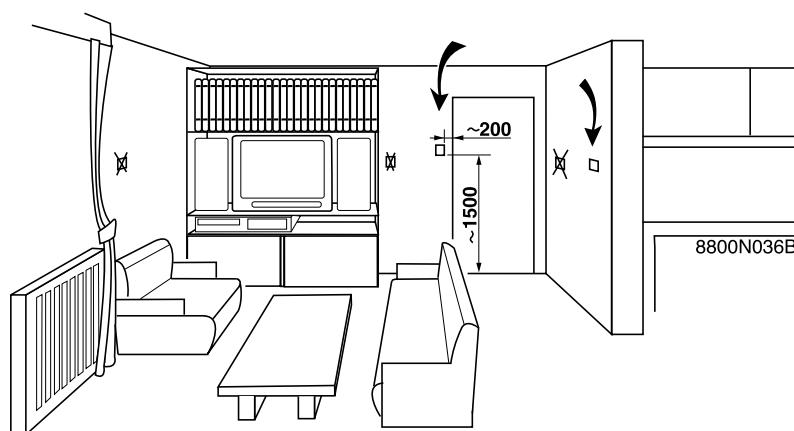
The remote control will be installed against an internal partition, about 1.5 m from the floor in a judiciously chosen "reference" room.
