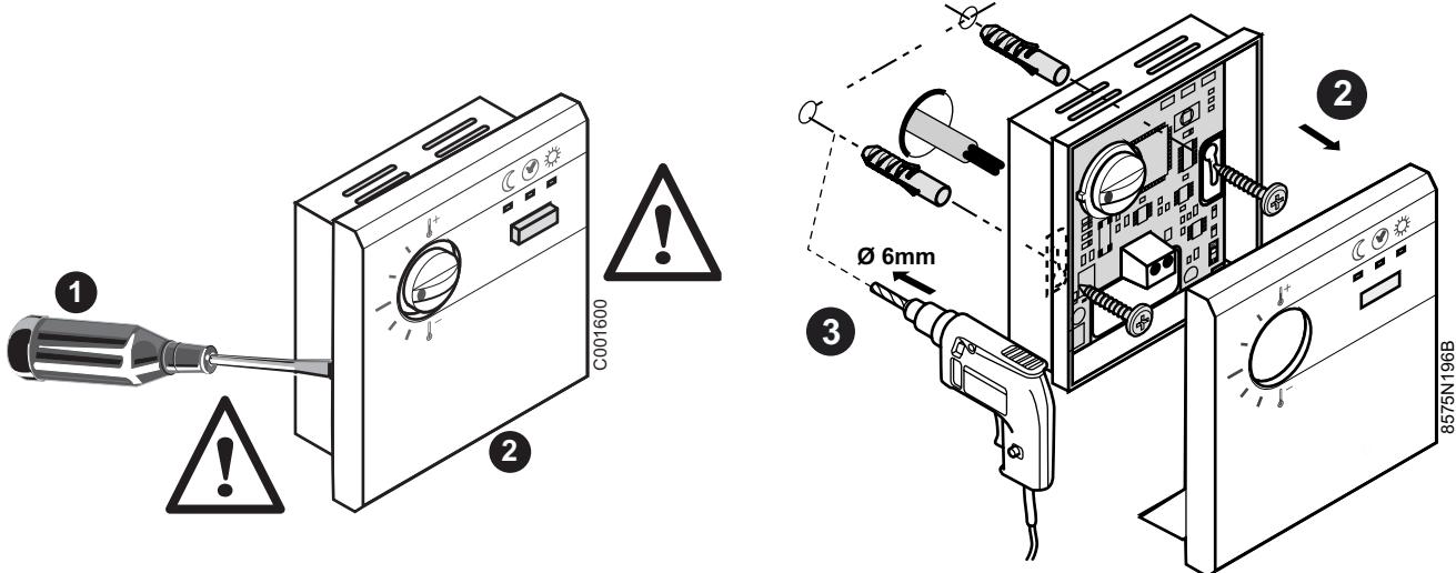
**⚠ ①** Carefully release the lugs on the front panel from the ribs in the box using a screwdriver.
