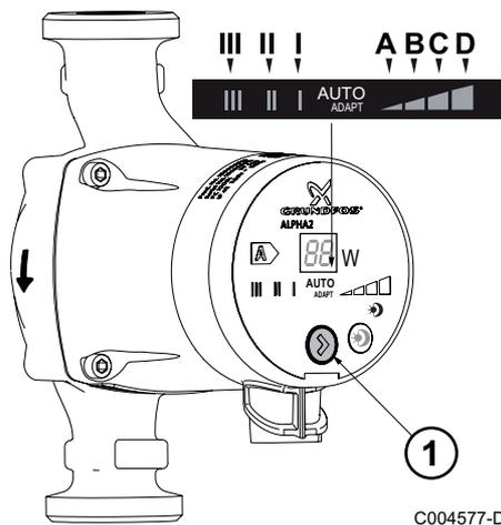
The pump is preset in the factory to position **AUTOADAPT**.
