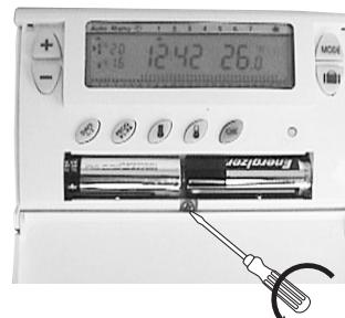
**1** Pull cover down and remove the screw.
