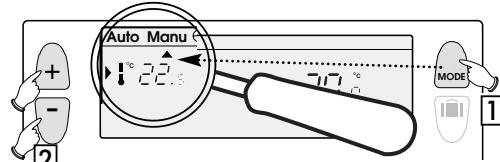
**1** Press the **MODE** button to position the pointer under **MANU**.
