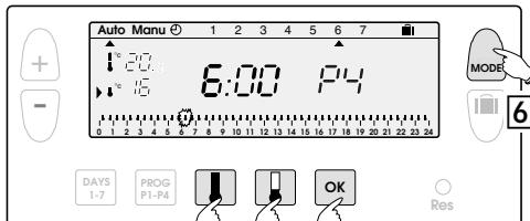
**4** Press the button several times to obtain **6h00**: the time to the wall displayed advances by 30 minutes for each short press. Continuous pressing accelerates the time run-off.
